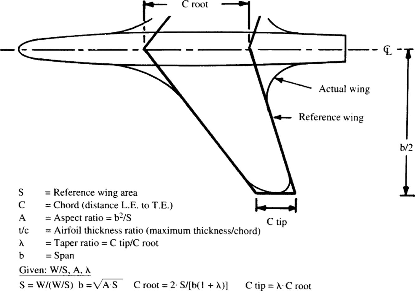
Fig. 4.15 Wing geometry.
