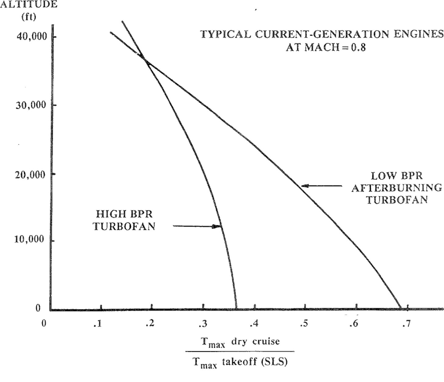
Fig. 5.1 Thrust lapse at cruise.
