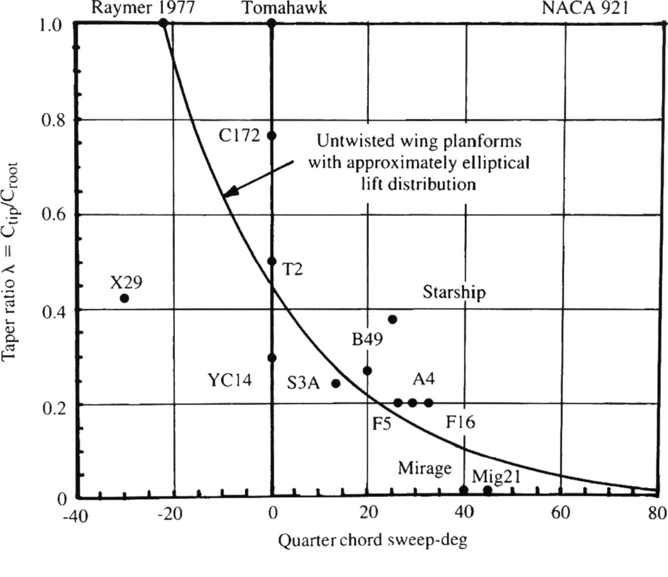
Fig. 4.24 Effect of sweep on desired taper ratio.
