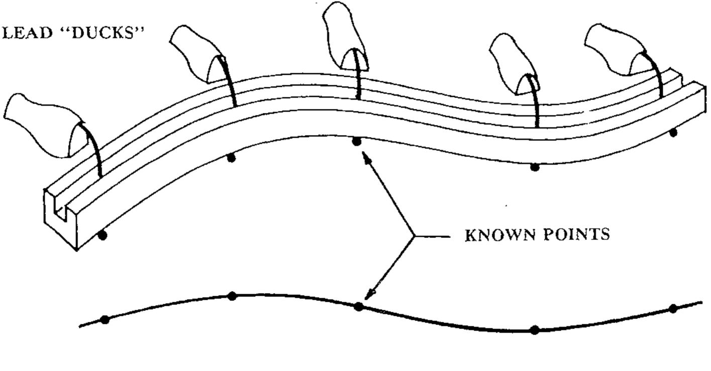
Fig. 7.9 Spline lofting.
