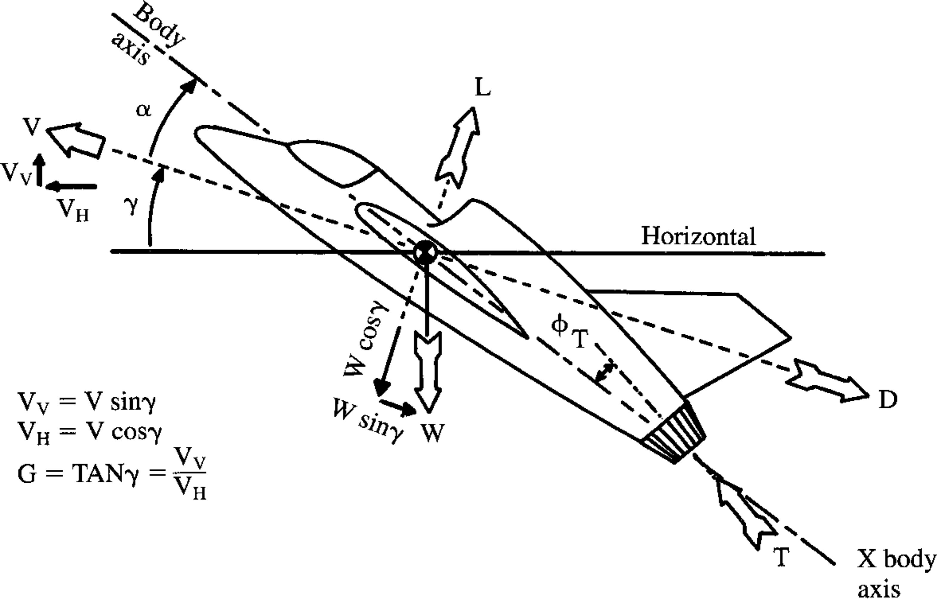
Fig. 17.1 Geometry for performance calculation.
