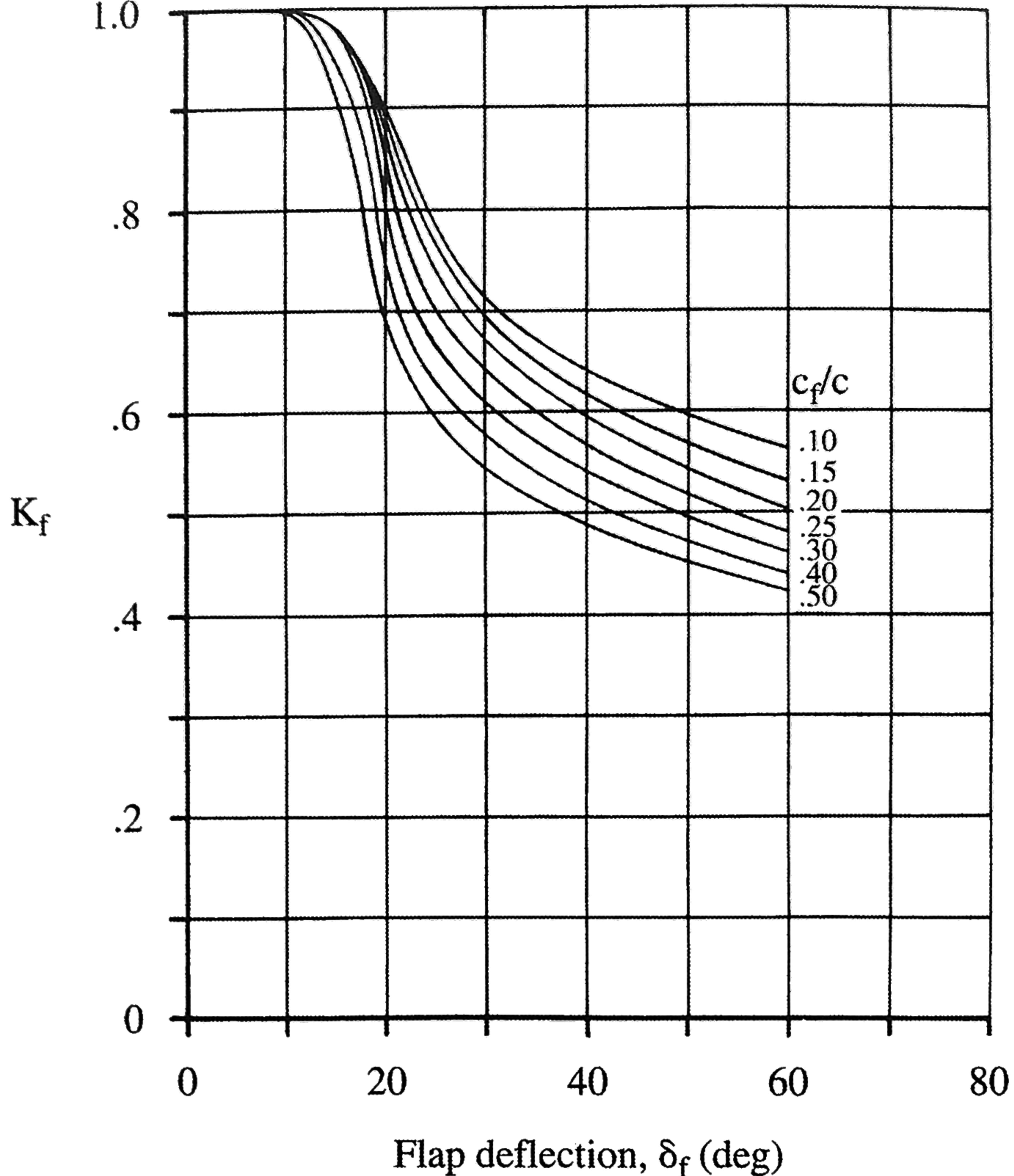
Fig. 16.7 Empirical correction for plain lift increment (Ref. 37).
