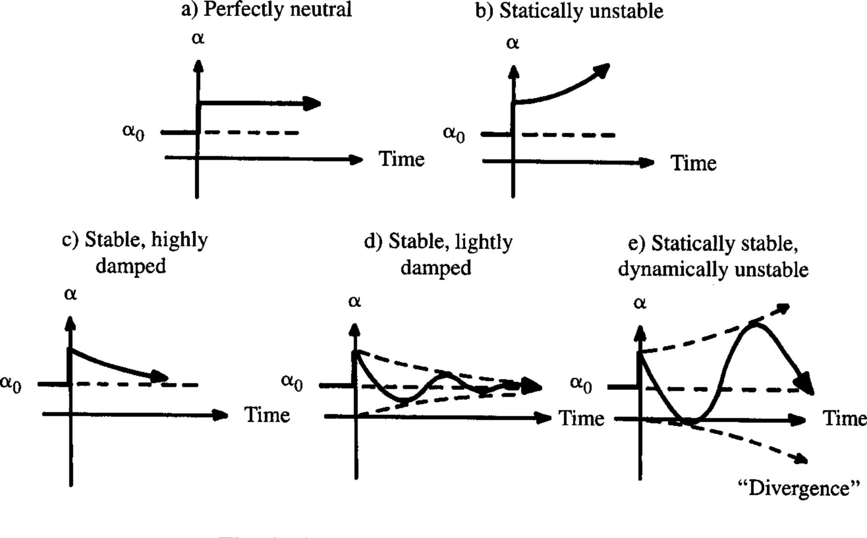
Fig. 16.1 Static and dynamic stability.
