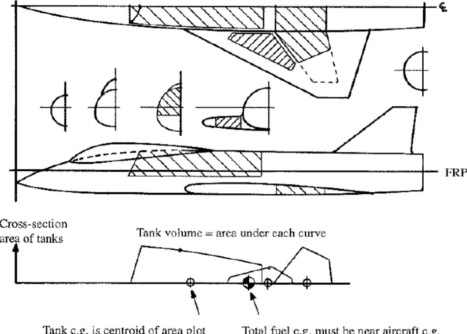
Tank c.g. is centroid of area plot Total fuel c.g. must be near aircraft c.g.
